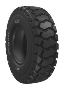
EARTHMAX SR 30 (E-3/L-3) is an *All Steel* radial tire which is dual-purposed for loaders and articulated dump trucks. The multi-layer steel belts and the rigid block pattern provide excellent traction, stability and durability. The special cut-resistant compound makes EARTHMAX SR 30 the ideal solution for a variety of harsh
