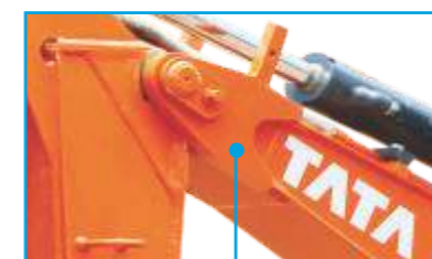
Reinforced boom end bracket
