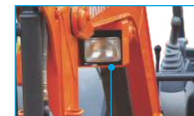
Compact boom lamp under the boom
