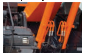
Strengthened boom foot
