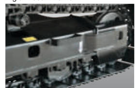
Strengthened track frame
