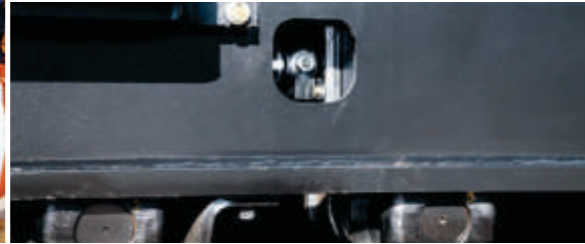
Adjuster greasing hole repositioned to reduce dirt accumulation
