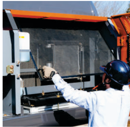
Easily detachable dust-proof indoor net
