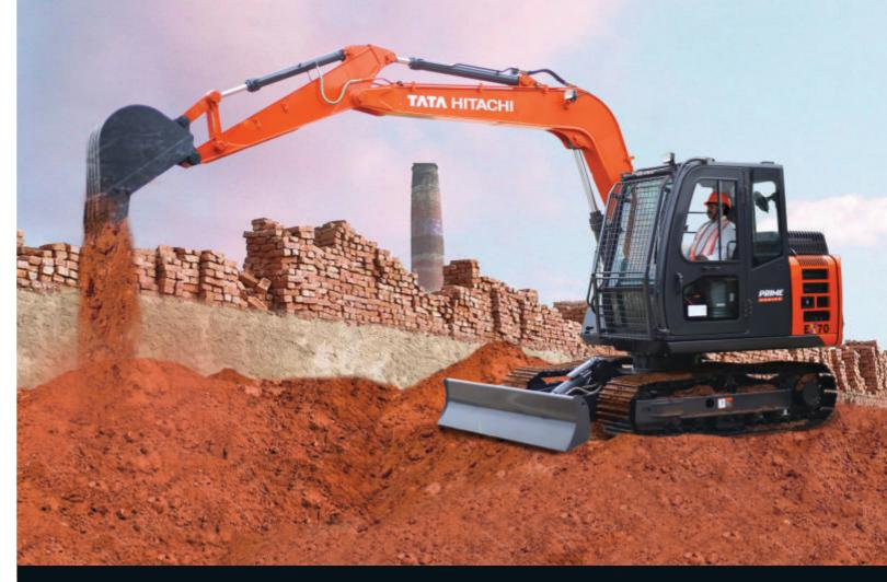
Model: EX70 | Engine Power: 49 PS @ 2000 rpm | Operating Weight: 7200 kg | Bucket Capacity: 0.13 - 0.68 m<sup>3</sup>
